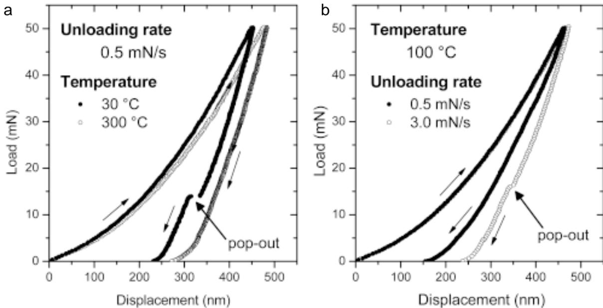
**Fig. 5.** Nanoindentation load-displacement curves produced on (111) silicon at (a) RT and 300 °C and (b) at 100 °C and loading rate of 0.55 and 3 mN/s using a Berkovich diamond indenter. The displacement discontinuity in the unloading curve (“pop-out”) is an indication of a phase transition during pressure release [22].
