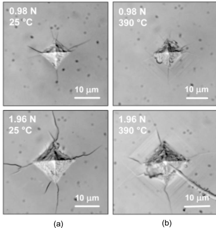
**Fig. 3.** Optical images of Vickers indentations produced on (111) silicon (a) at 25 °C and (b) 390 °C. Both imprints obtained at high temperature are surrounded by slip bands indicative of dislocation activity. Cracking around the indents was observed up to 550 °C.
