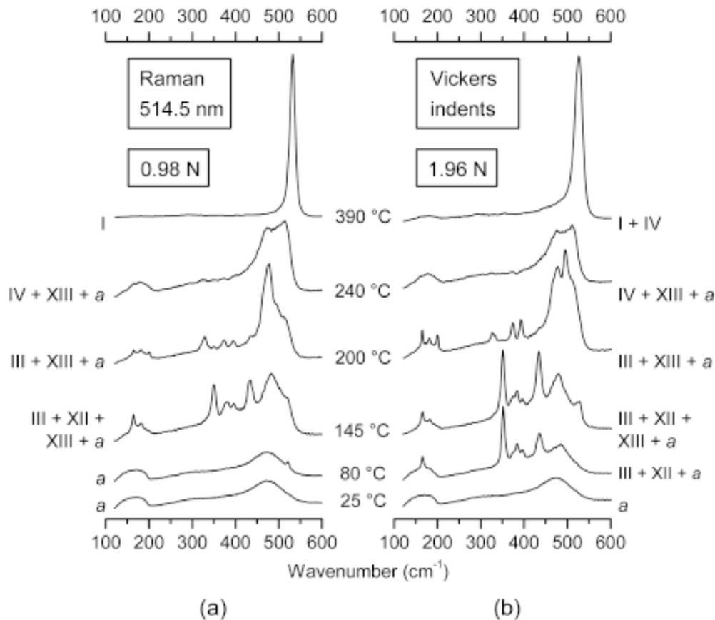
**Fig. 2.** Raman spectra of Vickers indentations on silicon produced at elevated temperatures under loads of (a) 0.98 N and (b) 1.96 N. Broad features at 160 and 480  $\text{cm}^{-1}$  indicate the presence of *a*-Si. The bands at 166, 184, 350, 375, 397, 435 and 485  $\text{cm}^{-1}$  are assigned to Si-XII and the bands at 166, 384, 415, 433, 465  $\text{cm}^{-1}$  to Si-III. Raman bands at 200, 330, 475, and 497  $\text{cm}^{-1}$  are assigned to Si-XIII [9].
