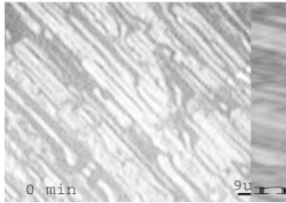
**Fig. 1.** Optical image of the as-quenched state of the freely solidified side of the Pd-based glassy ribbon.
