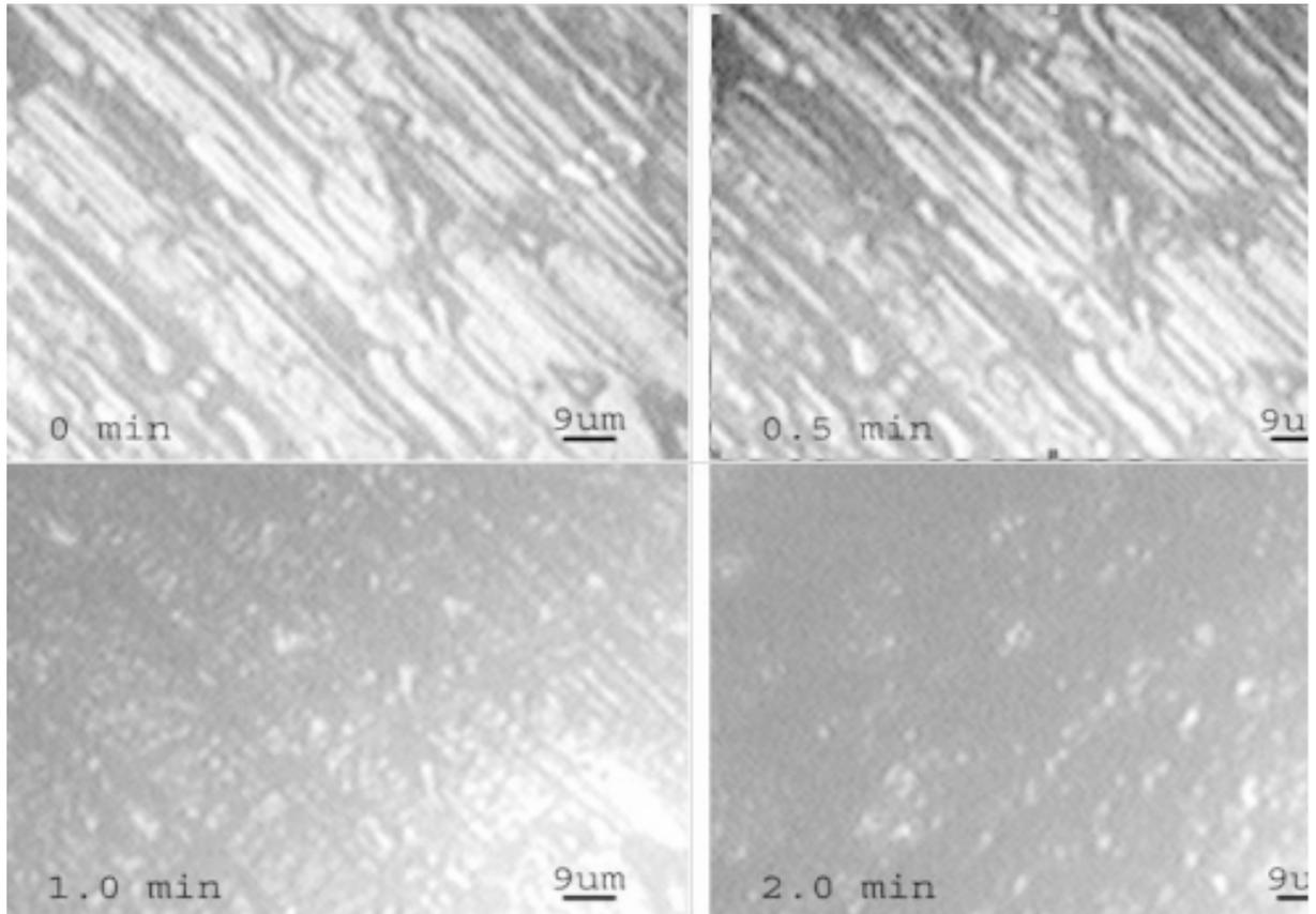
**Fig. 2.** Optical micrographs of the ribbon surface after various times at 583K; top left: 30 s; top right: 60 s; bottom left: 90 s and bottom right: 120 s.
